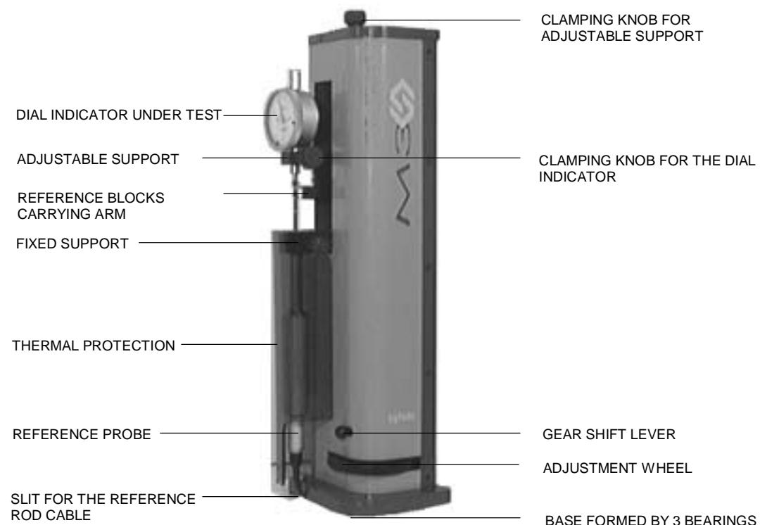
From experience, we built this support following ABBE's principle. By the fact, we minimize the alignment error.
